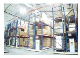
Installed on existing concrete slabs, our **ActivRAC** 16 Mobilized Storage System requires no costly structural footings or leveling. It's designed to articulate over reasonably unlevel flooring, while providing smooth operation.
